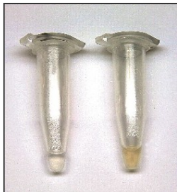
Figure 1. A blood sample extracted using DNA IQ™ (left) and Chelex® (right). Not all heme inhibition was removed by the Chelex® method. http://www.promega.com/applications/fnmrid/product_profiles/dnaiq
